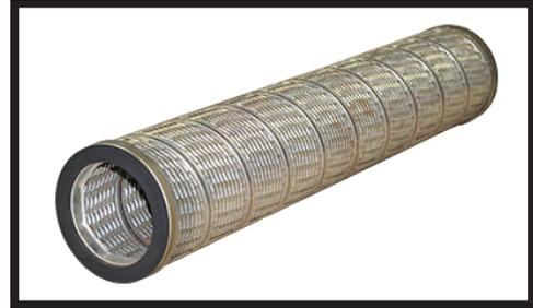
Providing a much greater surface area than a depth type filter, the pleated media cartridge is an excellent choice for expected high solids loading applications with the benefit of lower operating pressure drop and less frequent cartridge change-outs. For maximum efficiency these cartridges are rated to either 99.9% or 99.98% removal of 1 micron and larger solid particles.
