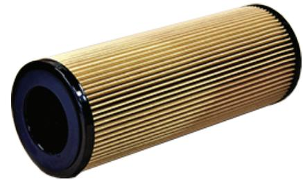
The media is treated cellulose and pleated for maximum surface area. The pleated media is supported by a galvanized or tin plated perforated metal core. A galvanized or tin plated metal end cap with bolt hole can cover one end as required for installation.
