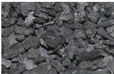
Activated Carbon Granules
