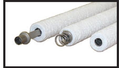
Fiber material such as cotton, polypropylene, or fiberglass is wound around a center core for the desired filtration needs. The core is offered in several materials to meet the application. Furnished separately, 304 stainless steel is the standard material for the installation hardware including the spring and cup assembly for the top hold down end and the post and pedestal for the bottom tube sheet end.
