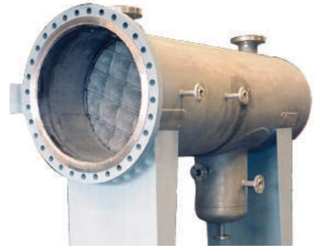
For each application the coalescer is designed for maximum dispersed phase liquid removal with minimal carryover. Variables which affect separation include velocity, viscosity, specific gravity, surfactants, and interfacial tension.
