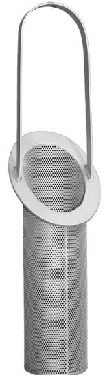
Dimensions are in inches. Tolerance is plus or minus 1/8". Strainer baskets have a 3:1 open area minimum with a standard perforated basket of 1/8" diameter holes on 3/16" centers. Perforated material is 40% open area.
